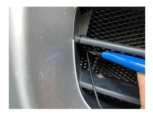
6. Now install the driver's side grille into the top opening of the bumper grille on the driver's side of the car.
