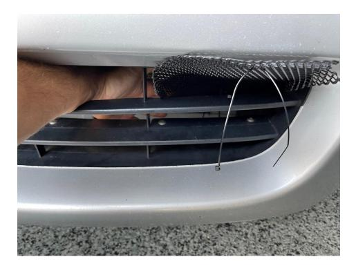
3. Then slide the grille, with the notch on the top left and the bends facing you. Slide the grille into position. The notch is to accept the aluminum bumper support on the top left (also on the driver's side). The grille will catch at that point. Continue to work the grille into position until the outer edge is contacting the rubber to the left. The flat end of the grille will line up with the center rib of the grille.
