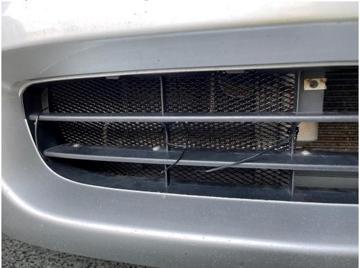
5. Ensure the flat end of the grille aligns with the center of the bumper grille center line. Then you can begin to snug the cable ties. Rotate the ends of the cable ties towards the face of the grille to hide the receiving ends. Then pull taught. You can then clip off the tails of the cable ties. The middle cable tie is there just for alignment. We will cut that one later and install a cable tie that ties both pieces together and also connects to the center bumper rib.
