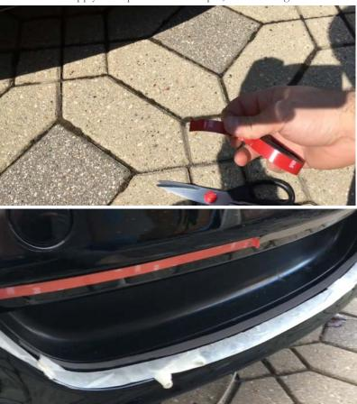
4. Once the tape is applied, position grill into tape. It may require pushing or pulling on the bumper cover to fit. You can use an allen wrench to pull the grill into position to hide the emblem tape as much as possible.
