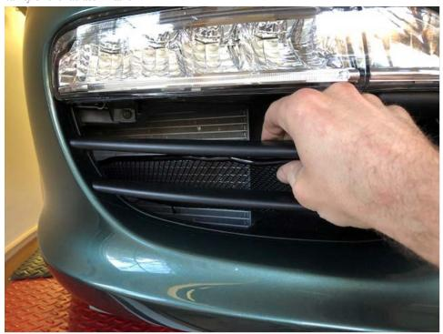
3. The hang up in the installation will be the outer most corner, it requires some work to get it past the black trim in the radiator cavity as shown in the left of the photo.
