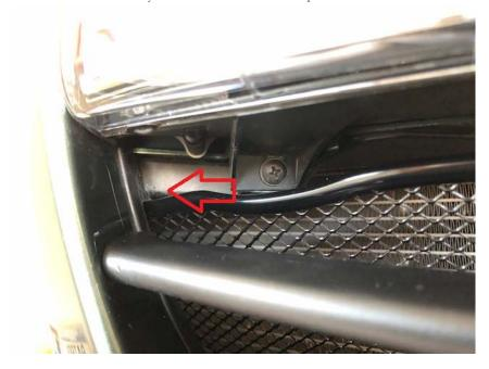
4. The cable ties can be hidden if you would like. The middle bar is two pieces. There are holes as shown in the next photos that the cable ties slip into. The receiving end of the cable tie will be on the bottom of the lower bar.
