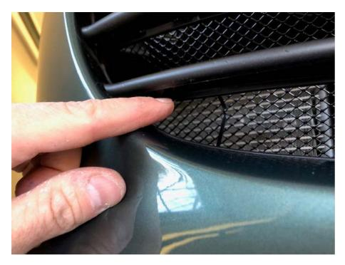
5. Pull the grille towards the front opening and align as you see fit. Should look like the photo below. Then using a side cutter, clip off the extra cable tie tail.
