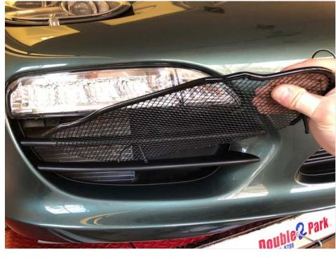
2. Cable ties are pre-installed for ease of installation. Insert hand into space above the middle rib. You will find that using your hand to guide the grille mesh to the outside of the car will assist with installation. Do not force the grille. Once the grille is inserted, you will be able to rotate the side in your hand into the cavity of the radiator intake.
