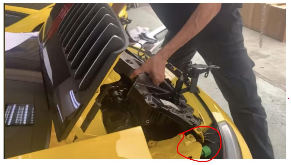
Slightly lift the clips marked in my picture, one on each side, to detach the spoiler base from the car body.
