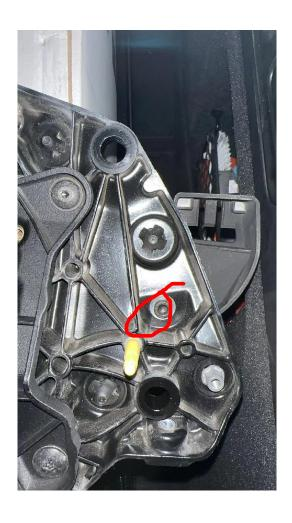
Install PartB as shown in the figure. Two screws on each side are tightened on the front and one screw on the side is tightened on the back. Use the six (6) 20mm M6 screws provided with the kit.
