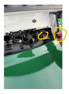
The brake light plug is connected like this.
