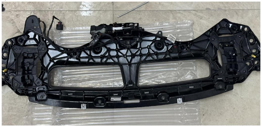
Install Part A on the tail base, with four screws on the left and right, and the four screws on the left and right that were removed before are just installed.
