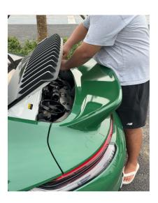
To affix the ducktail, use the two screws with the specification M6\*40mm. I have put it in the package. There are two screws in total, one on the left and one on the right. Tighten according to the position of the picture
