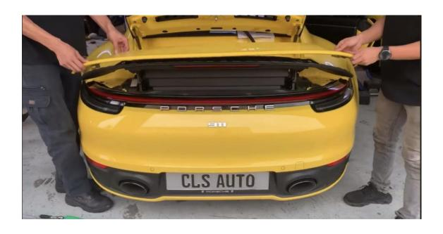
The top cover of the electric spoiler is secured by screws around it. Therefore, you need to remove the screws one by one as shown in the picture. After removing all the screws, two people can work together to remove the top cover.
