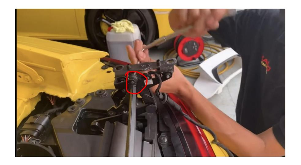
As shown in the picture, remove the screws that secure the upper part of the folding panel.
