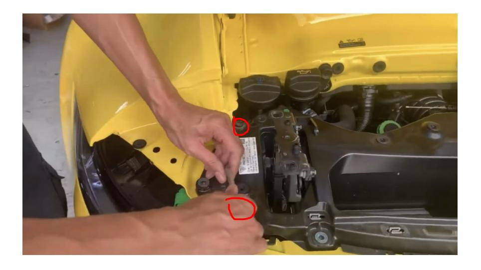
The spoiler base is secured to the car body by four screws, so you need to remove the two screws on each side one by one, as shown in the picture.
