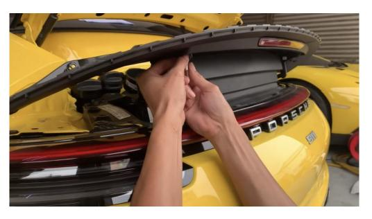
After removing the shield, we can take out the screws on the backside one by one, as shown in the picture.
