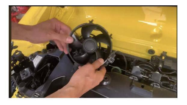
Use a screwdriver to remove the lower part of the folding panel from the clips Then remove the cooling fan to facilitate the movement of the tail base.
