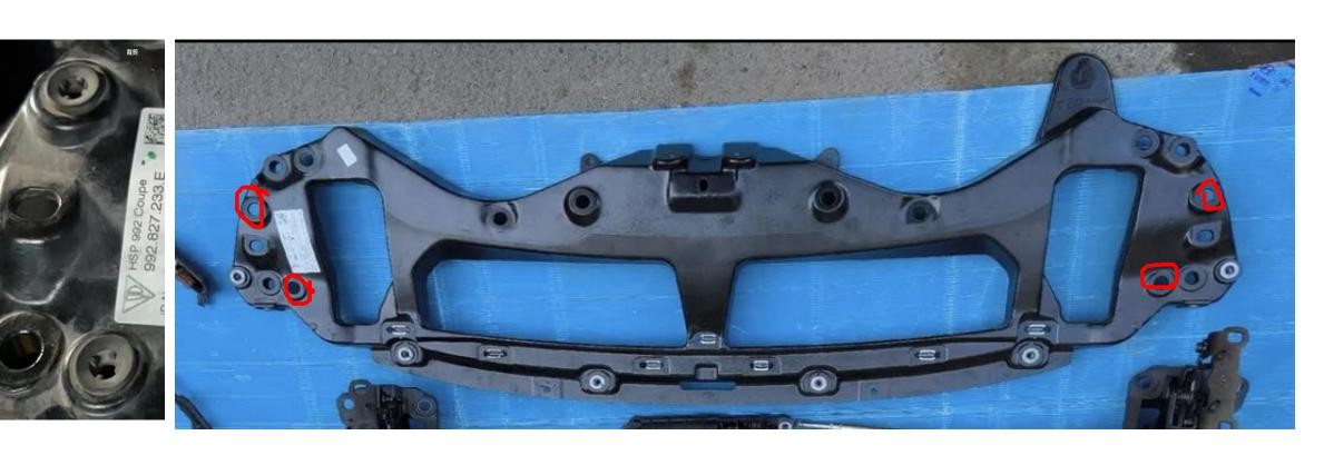
First of all, you need to remove these four rubber pads, two on the left and one, **be sure to remove them**!!! If they are not removed, the ducktail will sit too high.
