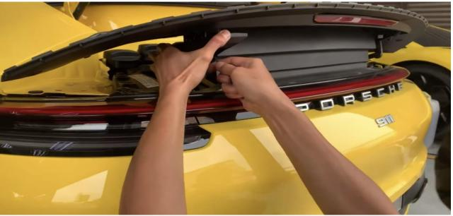
The screws securing the cover on the backside are protected by a shield, so we need to use a screwdriver to remove the shield first.
