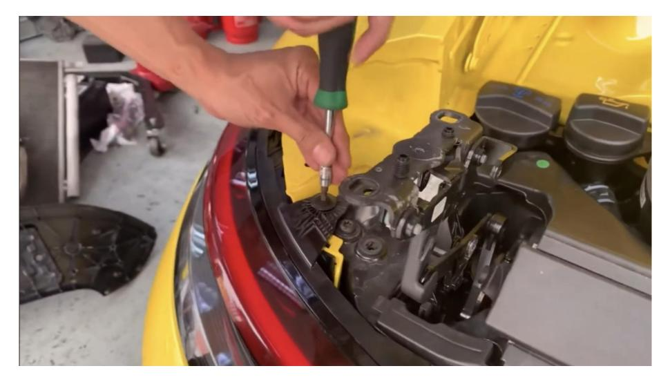
Remove the six screws that secure the taillights one by one.
