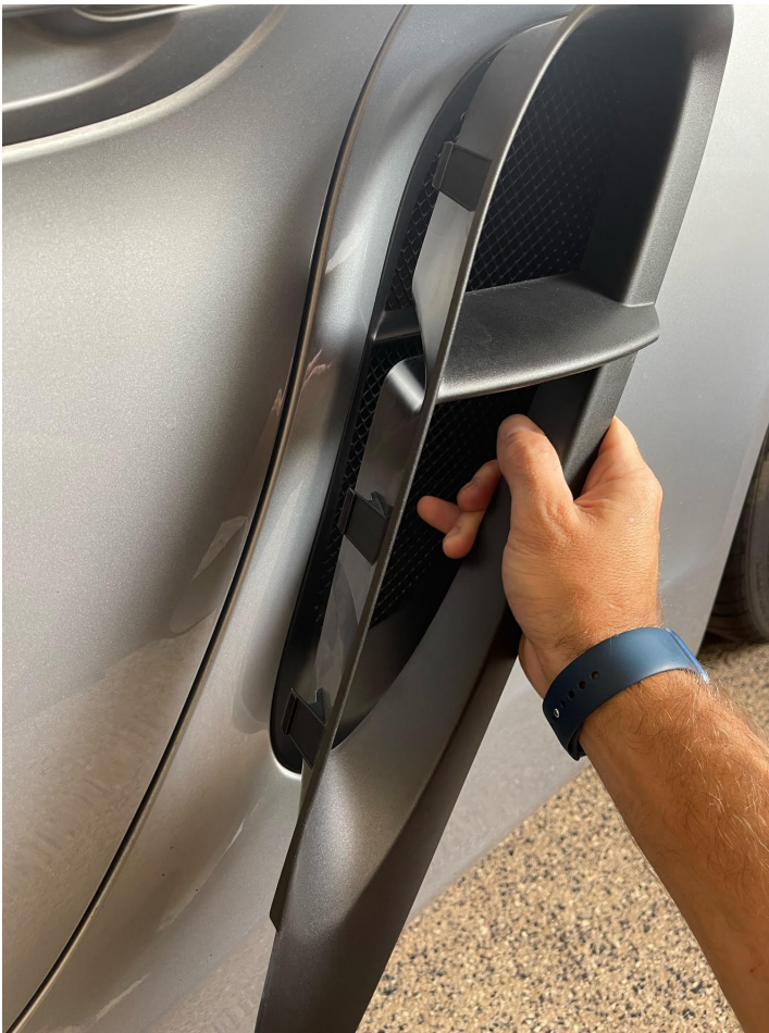
Inner edge of the 718 GTS side intake shown in position on a 981
