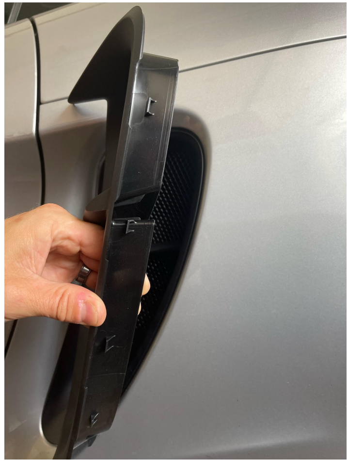
Outer edge of the 718 GTS Intake shown in position on a 981, clips are the same on all 718 side intakes.
